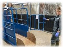
Open the back gate by lifting the latch and pulling the gate outwards.
